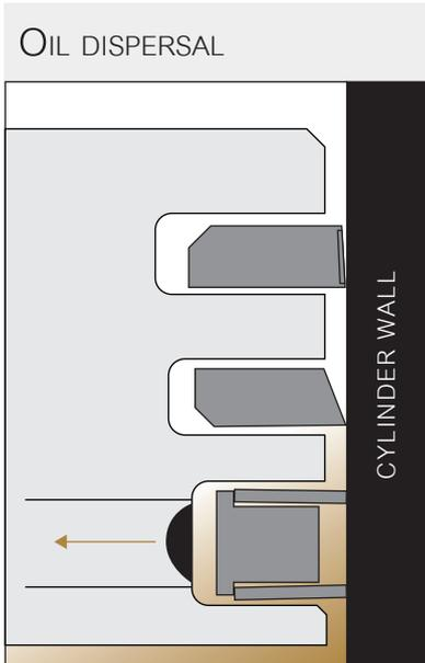
The bottom piston ring, the oil scraper ring, provides a nice thin layer of oil on the cylinder wall.
