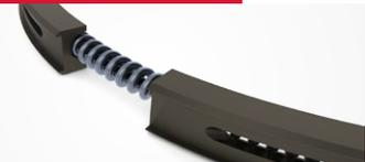
The oil control ring disperses and regulates the oil on the cylinder wall and scrapes the oil back down to the crankcase. This is necessary to ensure that the cylinder wall always has a thin, cooler film of oil from the crankcase. This guarantees that the friction between the piston and the cylinder is reduced so as to regulate the generation of heat.
