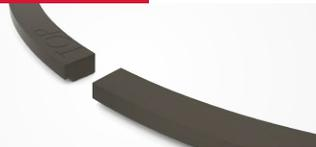
The scraper ring seals off the combustion gases, helps to dissipate the heat from the piston to the cylinder wall and lubricates and scrapes the oil from the cylinder wall towards the oil control ring. This prevents the oil from entering the combustion chamber.
